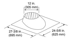
RF370 Roof Flashing
